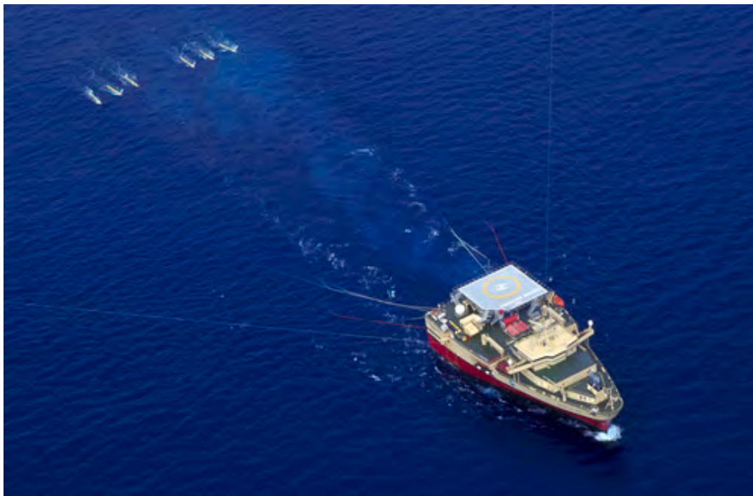
Figure 6. 3D Seismic acquisition offshore Guinea Bissau
