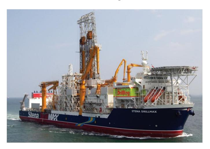
Stena DrillMAX is a state of the art, sixth generation, dual mast, dynamically positioned, deep water drill ship with extensive international and regional West African experience
